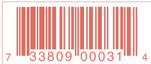
Figure 14.2 The bar codes on the goods we buy identify them. When the bar code is read by a computerised cash register (scanned), the computer supplies the price, which is then entered on the cash register tape. The code is read by template-matching on the basis of the positions, widths and spacing of the lines.
